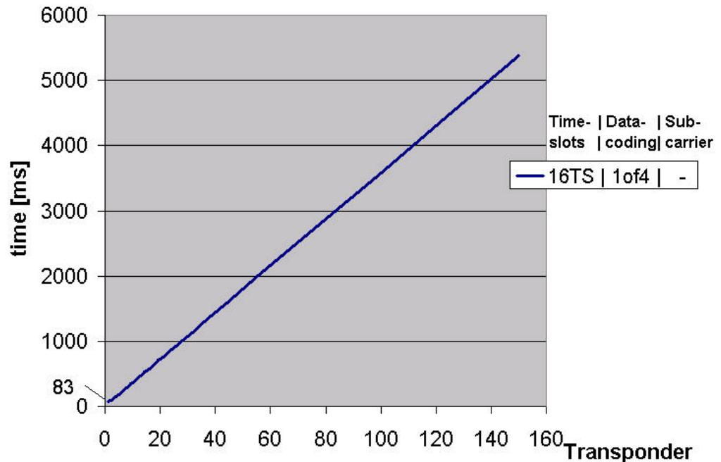
Please consider that the timing of the inventory command [0xB0 0x01] is influenced by the "More Bit". The "More Bit" is set if the number of transponders exceeds 24. If the "More bit" is set in the response of the reader to the inventory command, the communication time is influenced by the speed of the host system.
