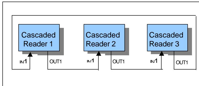
To set up Cascaded Synchronization, Buffered Read Mode must be enabled in configuration block CFG10: General System Parameters and Cascaded Synchronization must be selected in the SYNC setting in configuration block CFG11: Buffered Read Mode. The reader that should trigger the synchronization chain must be configured as MASTER in the SYNC setting in configuration block CFG11: Buffered Read Mode.
