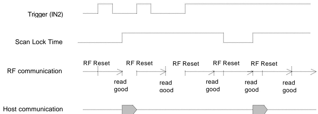
In continuous mode the reader sends data to the host, if new transponders were detected or the scan lock time for the transponders are over.
