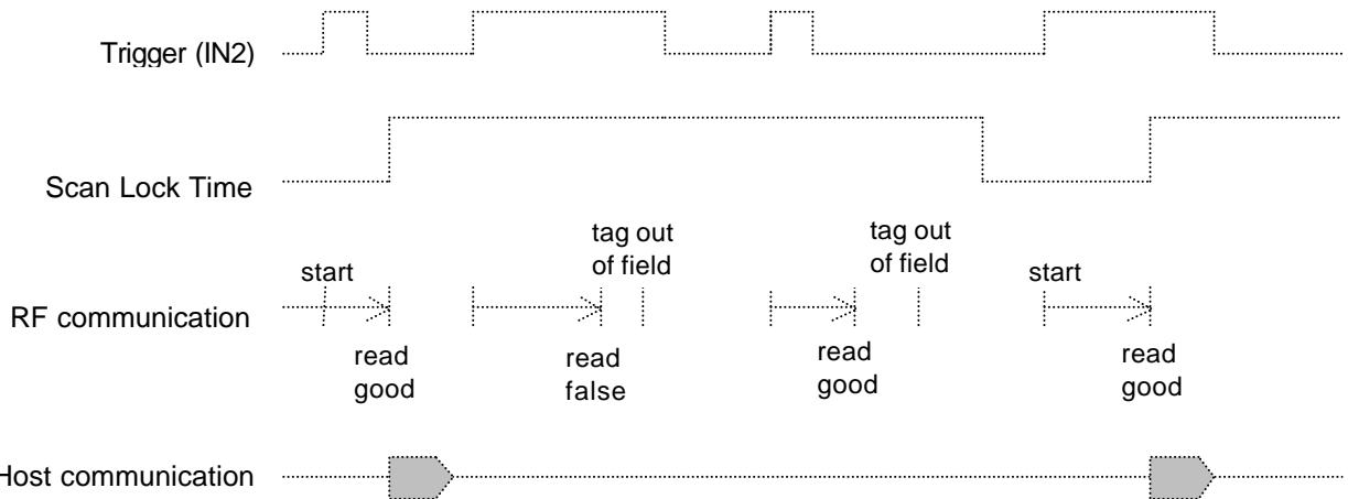
In single mode the reader only sends data to the host, if new transponders were detected or the transponders have left and re-entered the antenna field for the scan-lock-time.
