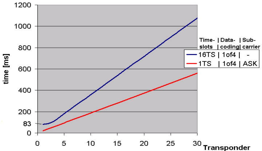
The measurement scenario for the average values is a worst case scenario where the transponders are static and close to the antenna. The results will be better if the transponders are moving or at different distances to the antenna.
